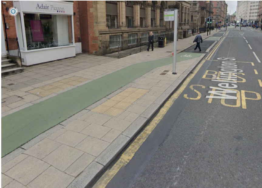
Figure 4: Reduced-width Bus Stop Bypass
